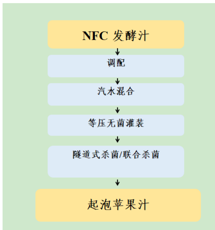
Figure 8-2 sparkling apple juice production process
